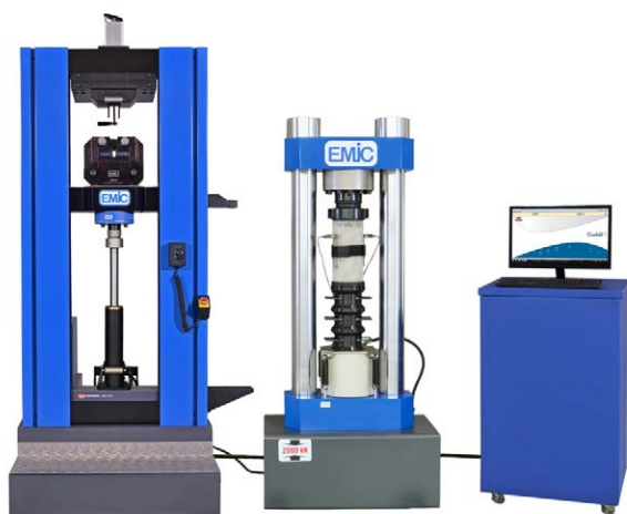
SISTEMA 200/2000: 23-200 + AC6.08 + DP1.23 + BH3 C/ TEST PROFILER
